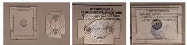
The fluidic component and the support are made of transparent resin
