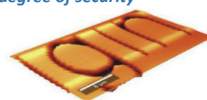
AFM image of security element type nano-text on the surface of the smart hologram
