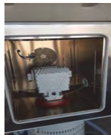
Fig. 12b. - Vibration system with camera climate (Frequency band: 2000 Hz. Maximum mass of the device tested 50kg)
