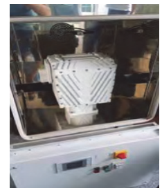
Fig. 12c. – Climate room for environmental testing (temperature: -40 °C/+180 °C; humidity: 10-95% RH)
